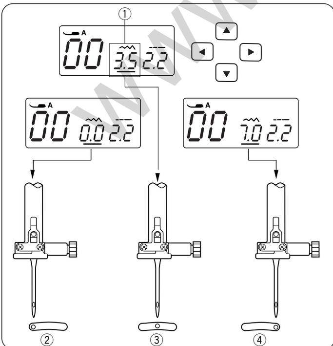
**• Adjusting the needle drop position**
