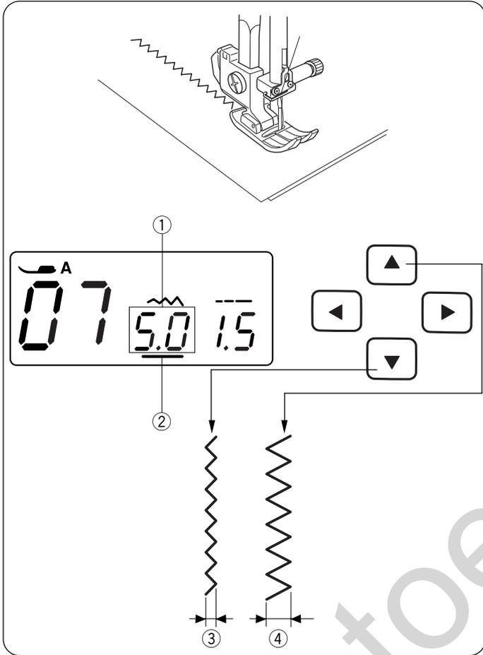
The zigzag stitch is one of the most useful and versatile stitches. It is used for overcasting, mending, appliqué, and also used as a decorative stitch.
