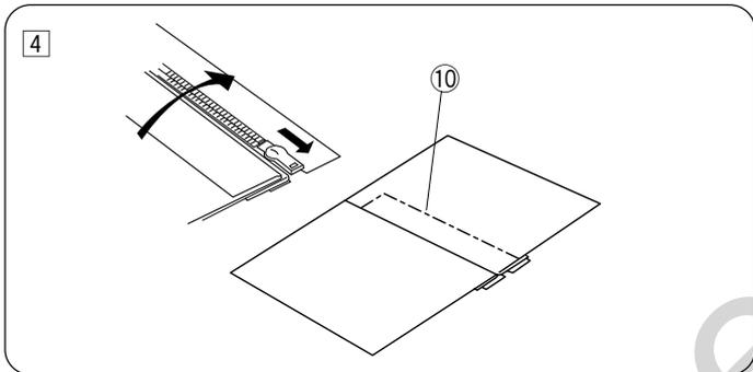
4 Close the zipper and open the upper fabric flat over the zipper. Baste the upper fabric and zipper tape together.
