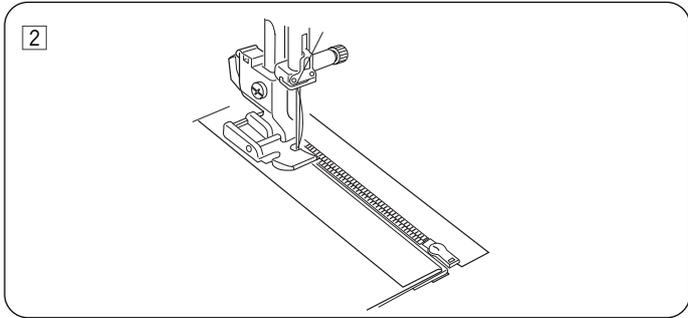
2 Attach the zipper foot with the pin on the right. Sew through all the layers from the end of the zipper opening, guiding the zipper teeth along the edge of the foot.
