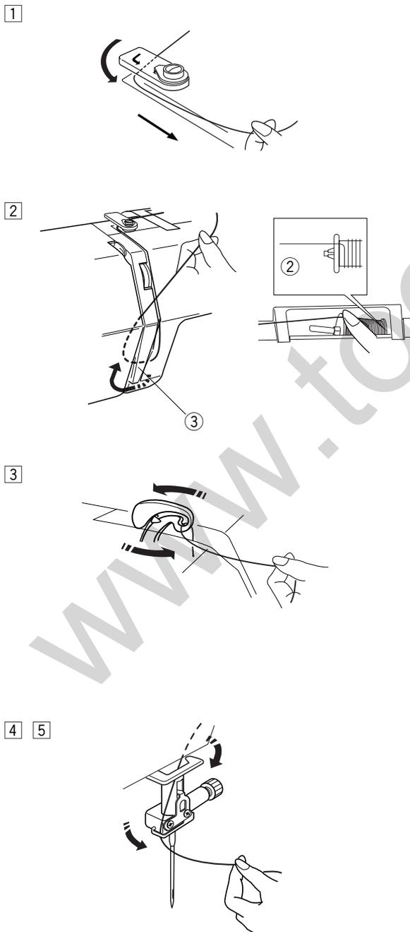
① Draw the end of the thread around the upper thread guide.
