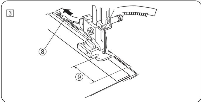
3 Stop the machine 2" (5 cm) before the foot reaches the slider on the zipper tape. Lower the needle into the fabric, and raise the foot. Open the zipper, then lower the foot and stitch the remainder of the seam.
