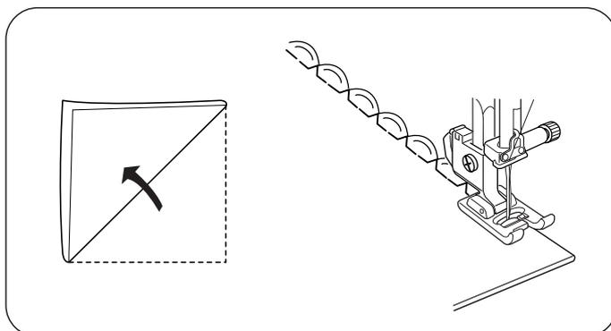
Use a lightweight fabric (tricot, for example). Fold the fabric as shown and stitch on the fold. Allow the needle to just clear the folded edge to create a shelled edge. You may need to increase the needle thread tension slightly.
