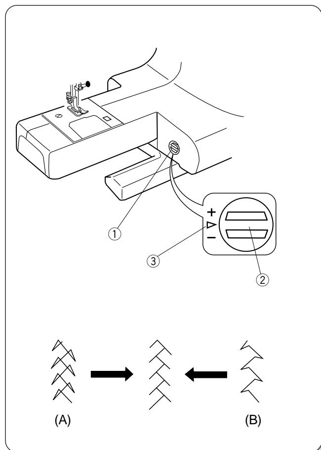
The sewing results of the stretch patterns may vary depending upon the sewing conditions, such as sewing speed, type of the fabric, number of layers etc.
