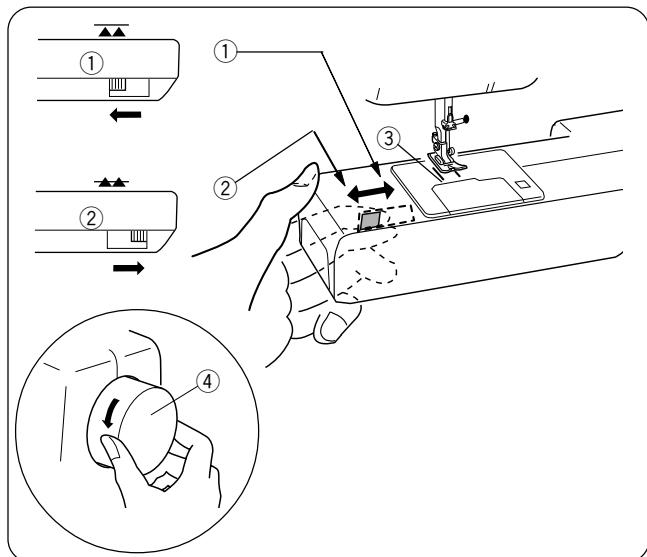
The feed dog can be lowered with the drop-feed lever for sewing on buttons etc.
