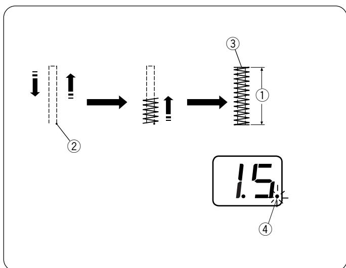
Tacking is used to reinforce pockets, crotches and belt carriers where extra stretch is needed.
