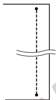
Lower the needle close to the front edge of the fabric and lower the presser foot. The machine will sew several locking stitches in place and continue sewing forward. By pressing the reverse button ④, the machine will sew several locking stitches in place, then stop sewing automatically.
