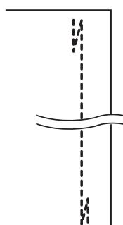
This reverse stitch can be used for securing, mending or reinforcement stitches. At the end of seams, press the reverse stitch button ④ once, so that the machine will sew an auto-lock stitch immediately and stop automatically
