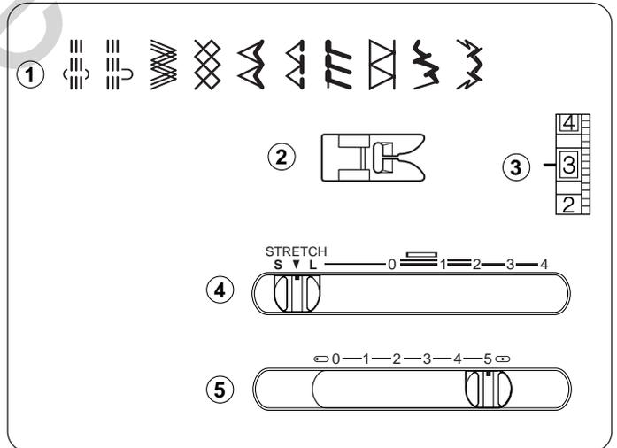
If forward and reverse feeds become unbalanced due to the type of fabric, adjust the balance by sliding the stitch length control as follows:
