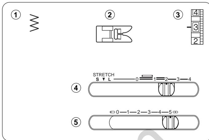
Simple zigzag stitching is widely used for overcasting, sewing on buttons etc.
